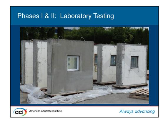
Testing for Phases I and II were performed on 6 ft. x 6t ft. ICF wall sections like the ones in this photo.
