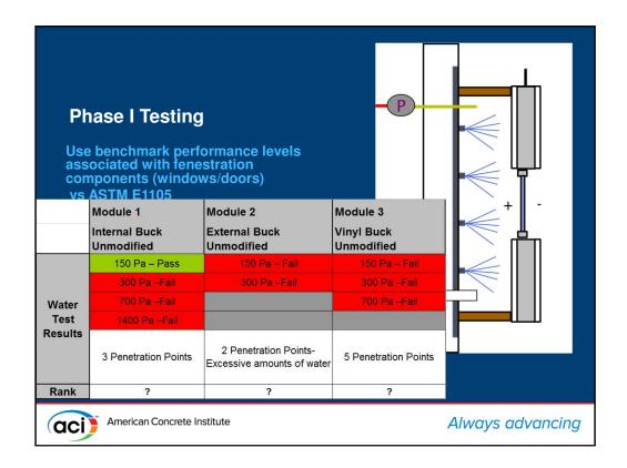
The consulting engineers for the project, RDH Building Science, suggested that the test criteria be borrowed from the fenestration industry, which is required to test their products to varying performance levels, according to climate conditions and building use, or ASTM E1105.
