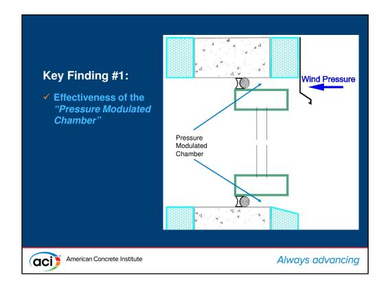
Now, as we view the installed window assembly, the space between the window and the structure becomes the pressure modulated chamber, with the rod and caulk at the back creating the seal.
