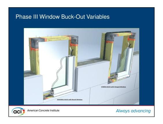
These photos give a sense of how the openings were prepared for the examples where the forming materials were left behind.
