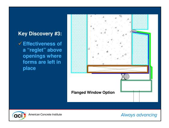
Since the industry was quite insistent on a "flanged window" option, we did successfully test that with an added head flashing that extended over the window flange.
