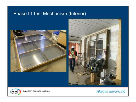
A pressure chamber was set up on the interior, which was intended to pull water through the assembly at carefully monitored levels of negative pressure.
