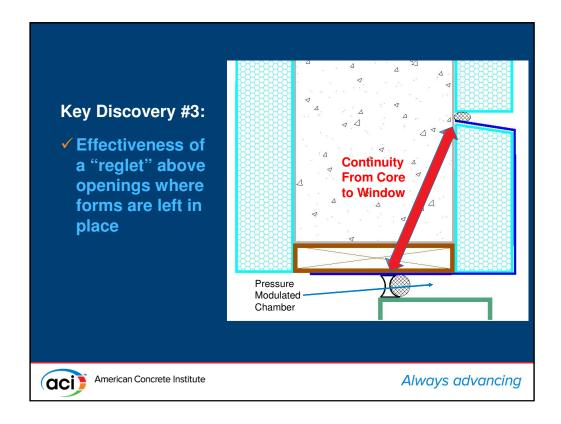
The third key finding was the effectiveness of an ICF-specific adaptation of through-wall flashing, which we are calling the "reglet" technique.
